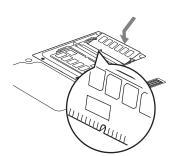
Figure 4-8. Installing a Second Memory Module
